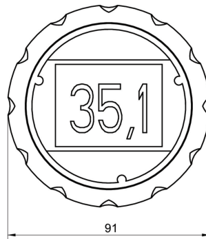
FlexHousing front view
