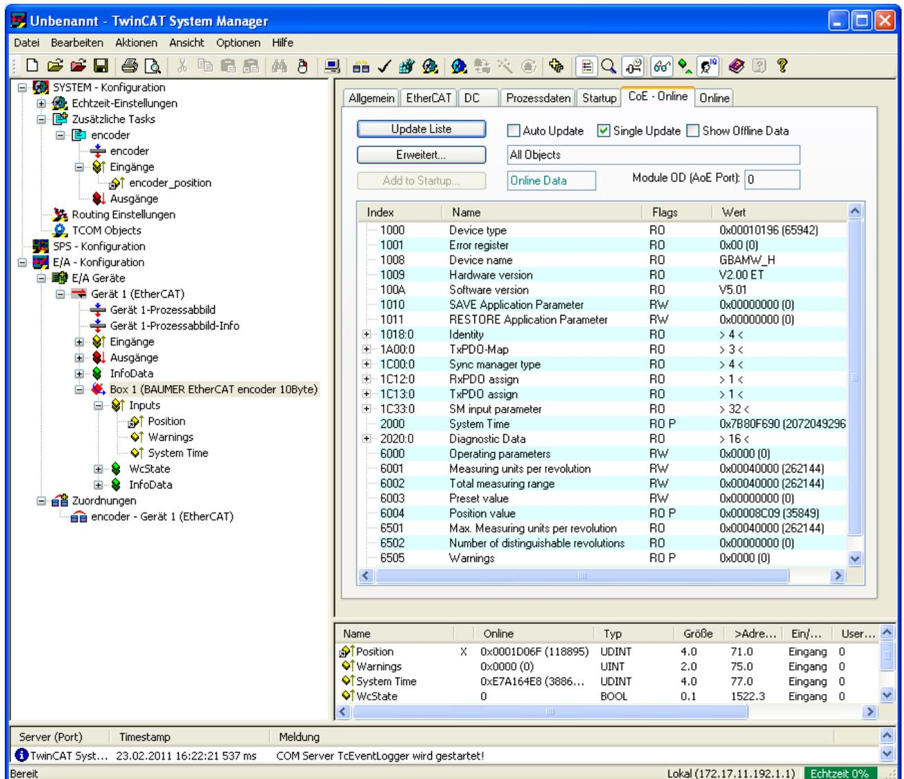
The screenshot displays the TwinCAT System Manager interface. The left-hand tree view shows the project structure, with 'Gerät 1 (EtherCAT)' expanded to show its configuration, including 'Box: 1 (BAUMER EtherCAT encoder 10Byte)' and 'Inputs'. The main window is titled 'CoE - Online' and contains a table of SDO objects.
