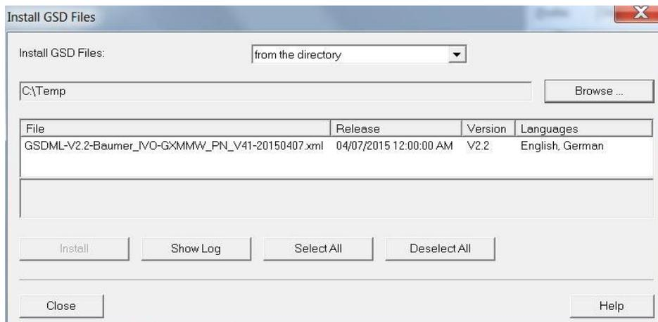
The encoder appears in the hardware catalog at the right under „PROFINET IO“ – „Additional Field Devices“ – „Encoders“ – „Baumer IVO PROFINET Encoder“ - “Baumer IVO PROFINET Encoder” – „GxxMW” (“xx” depending on encoder).
