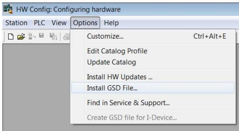
In the following dialogue please select the directory including the GSDML file. Mark the file on screen. „Close“ will finalize the operation. The same directory also includes the corresponding Bitmap file providing a small encoder image in the engineering tool. This file is automatically installed in parallel.
