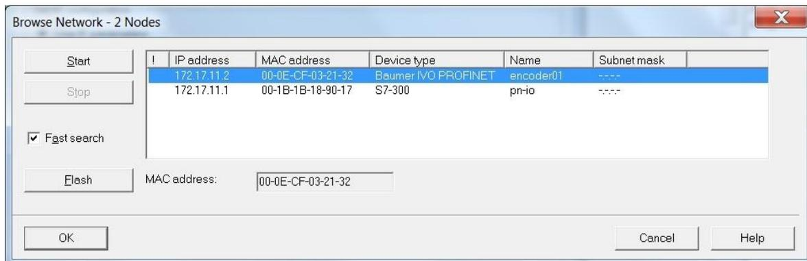
The MAC address serves as a unique identifier. When clicking the button „Flash“ the highlighted device will flash its status-LED so it can be found easily amongst other devices.
