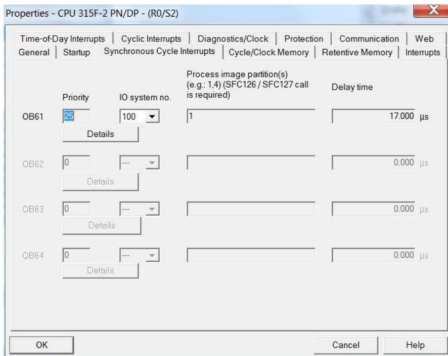
A click on button „Details“ provides OB61 properties assigned sub-process image 1.
