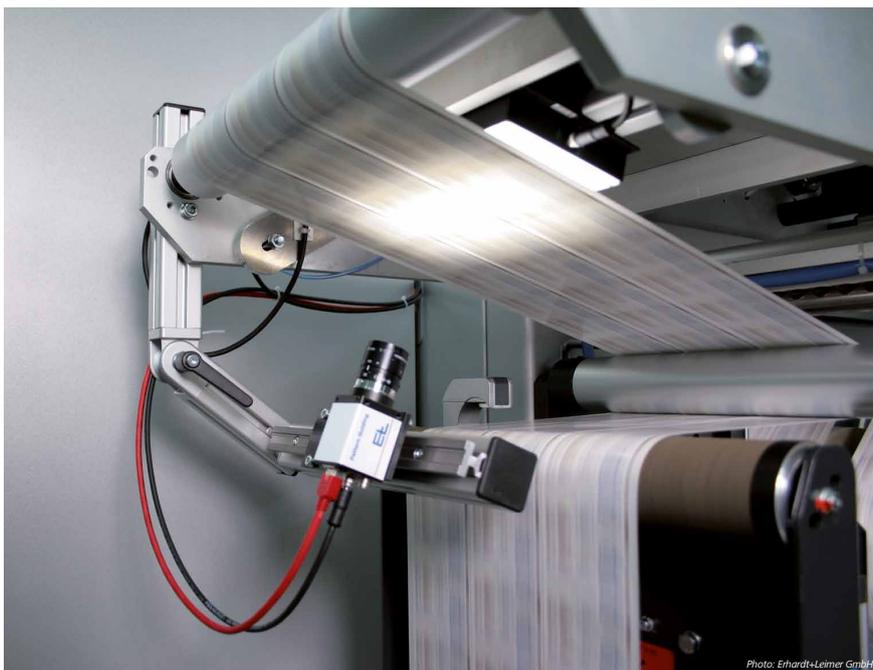
The ELCAM „Cut-to-Mark“ system makes sure the label web is precisely guided in the cutting process.
