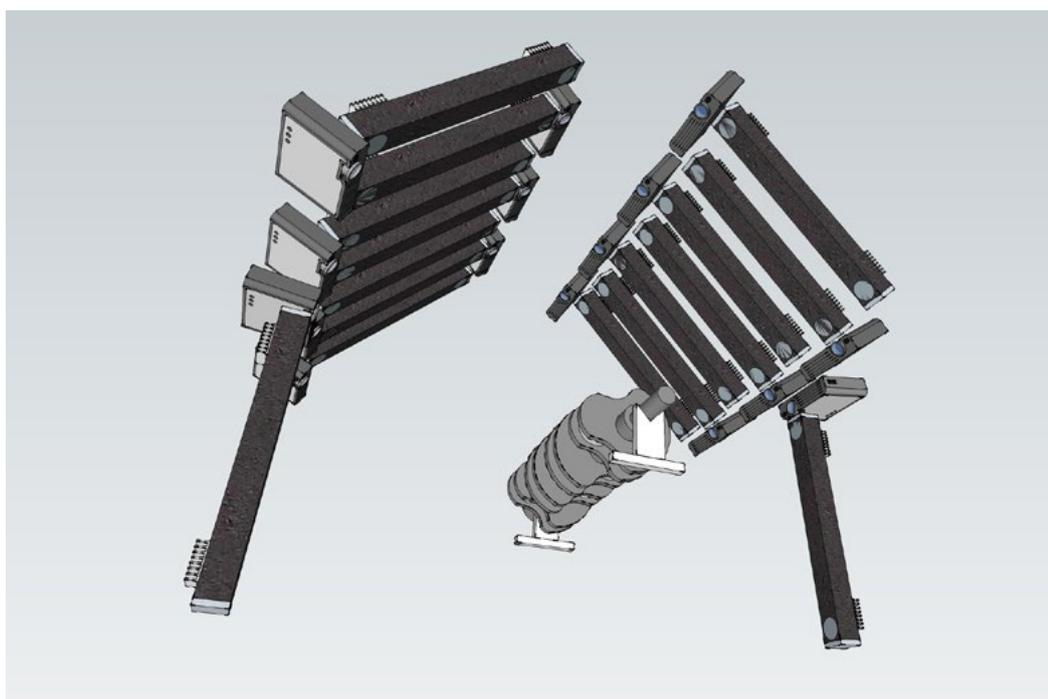
The image processing-based system comprises 16 carbon-fiber arms, each one holding two VGA Baumer cameras and a LED video projector. The system can be flexibly adapted to the size or complexity of a crankshaft.
