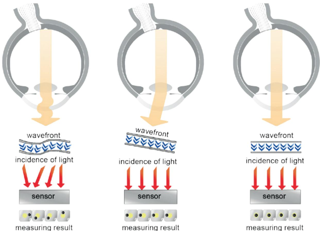
*In wavefront analysis the generated pixels (black dots) are compared with the reference points of an ideal imaging lens (yellow points).*
