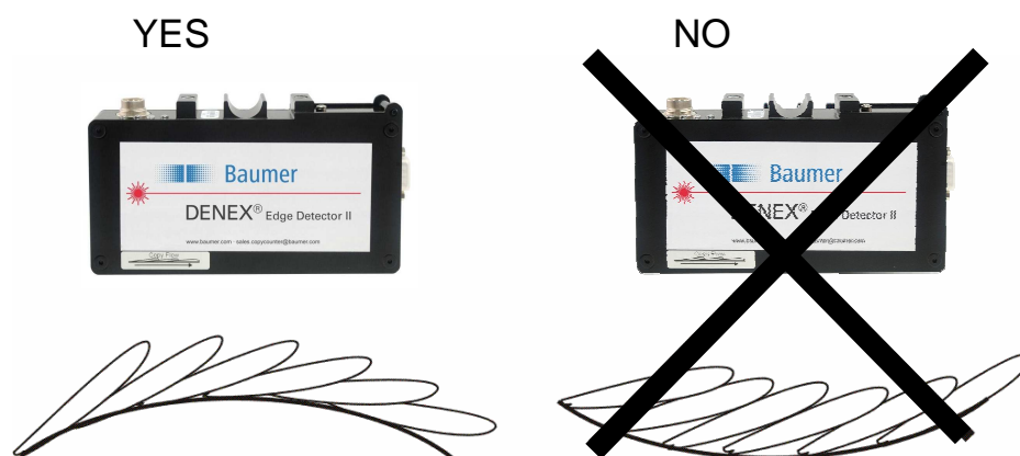
Figure 3.2.1 Mounting on a non-flat conveyor.
