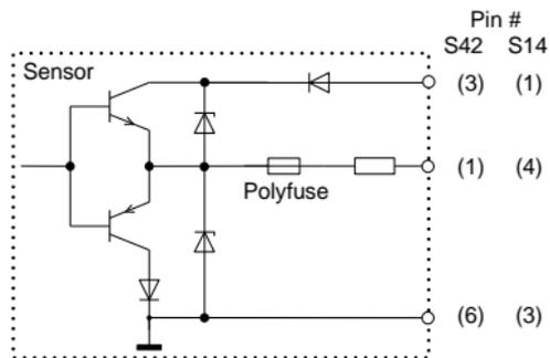
$+V_S$  Operating voltage (+10VDC ... +30VDC)
