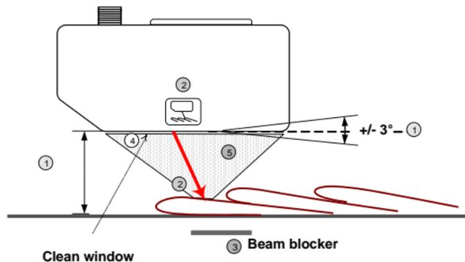
Line focus perpendicular to the **Scatec** housing
