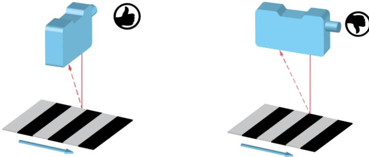
In the correct orientation, the influence on the measuring accuracy is low. In the wrong orientation, the deviations depend on the differences in reflectivity of the various colors.
