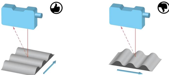
If the contour of an object is measured, it is important to ensure that the object moves at right angles to the sensor, to avoid shadowing and reflections on the receiver.
