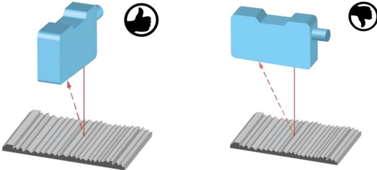
Particularly with shiny objects, for example turned parts, ground surfaces, extruded surfaces and the like, the installation position affects the measuring result.
