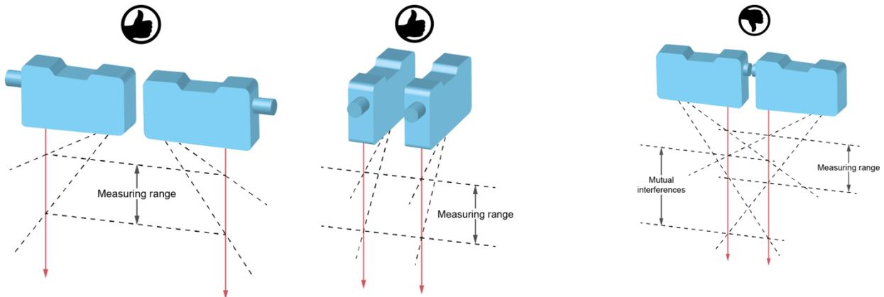
If several optical sensors are used, they may mutually influence one another. During installation, ensure that only the sensor's own laser spot is in the detection range of the receiver. Up to a measuring range of 600 mm, the sensors can be lined up in a row without them influencing each other (picture in the middle). If the mutual interference cannot be avoided through installation, the sensors can be operated asynchronously using the Sync-In input, see chapter TRIGGER MODE.
