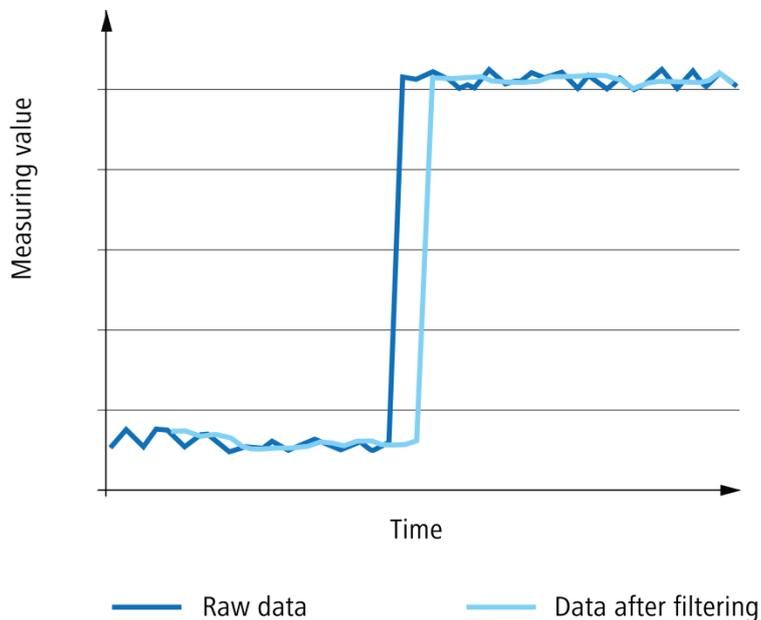
This diagram shows the effects of the median (number of measured values 5). The filter is used to suppress measurement errors. The output only changes after a defined number of measured values (number of measured values/2). The measuring frequency is not affected by this filter, but the response time is.
