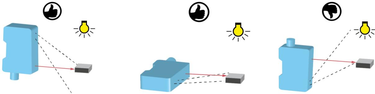
When installing optical sensors, it is important to ensure that there is no strong ambient light in the area of detection of the receiver.
