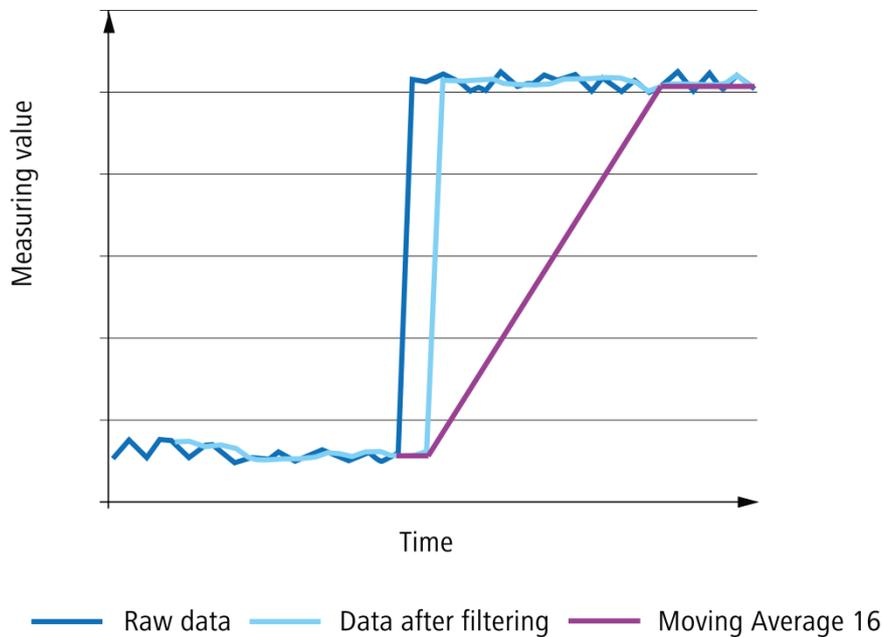
As shown in the diagram, the moving average evens out the output value. In contrast to the median filter, it is possible that with the moving average, the displayed measured values were never measured as such. The measuring frequency is not affected by this filter, but the response time is.
