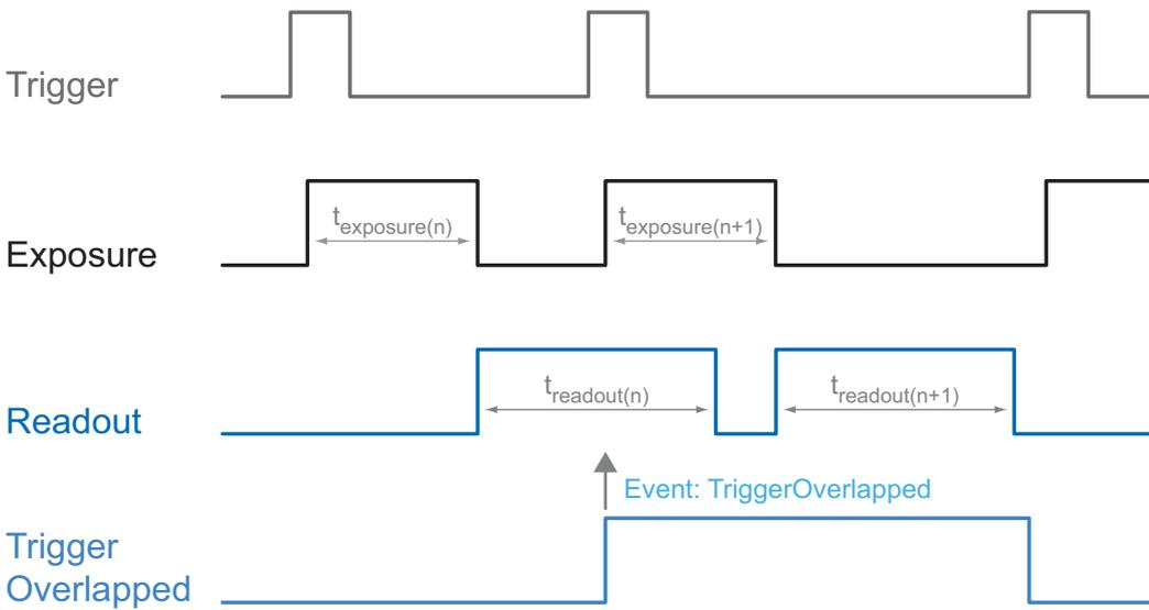
Once a valid trigger signal occurs not within a readout, the "TriggerOverlapped" signal changes to state low.
