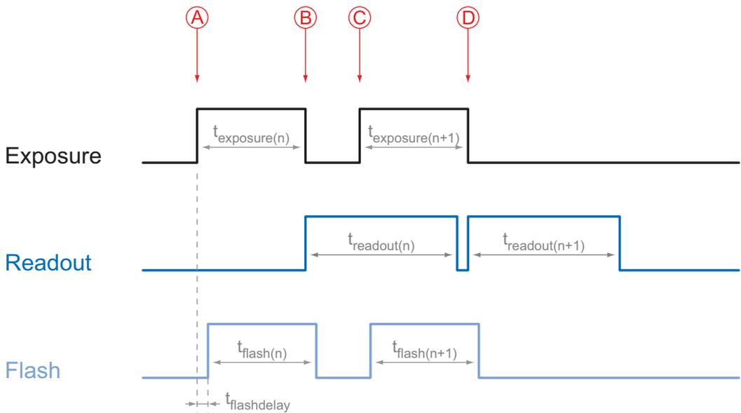
$$t_{\text{flash}} = t_{\text{exposure}}$$
