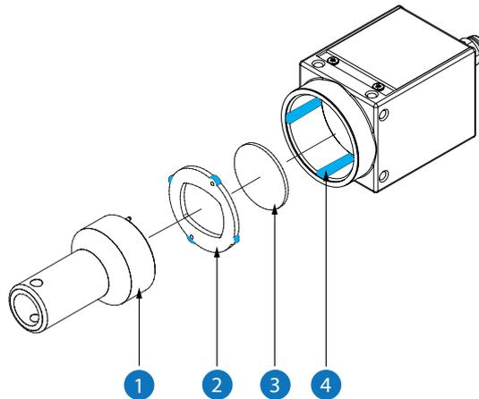
1. Insert the assembly tool (1) into the sensor opening. Place the two pins at the front end into the locator holes of the filter holder (2).
