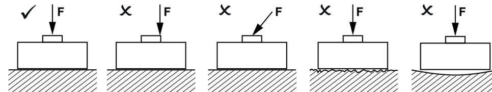
Force is to be applied centrally in axial direction.
