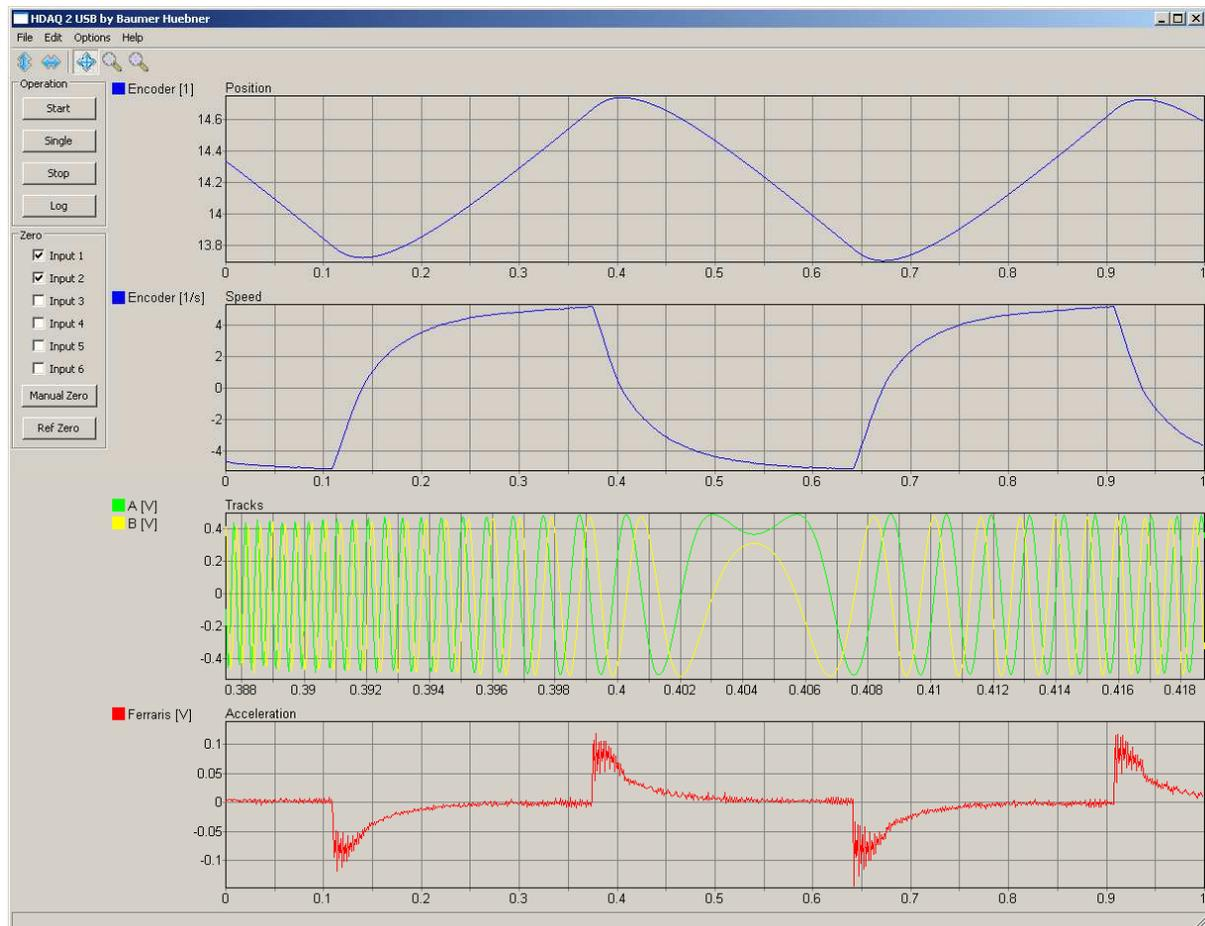
**Figure 16: Example data captured from a sine/cosine encoder and a Ferraris sensor**
