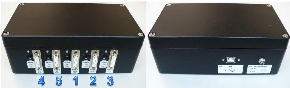
**Figure 1: a) Encoder inputs**
