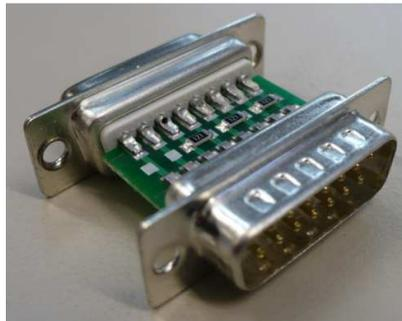
Figure 3: Terminating resistor adapter
