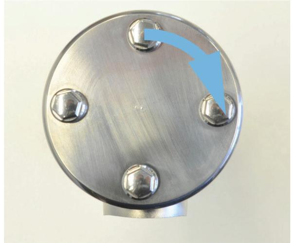
4. Tighten the screws crosswise only so far that the light blue cover seal is flush with the surface of the housing.
