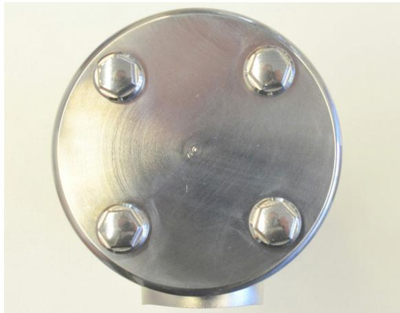
To do this, loosen the 4 screws by approx. 1.5 mm (2 turns).
