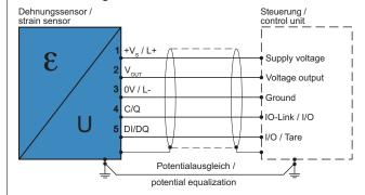
Output signal:  $V_{OUT} = \pm 10 \text{ V}$ , parameterizable Operating voltage range: +Vs = 18 to 30 VDC
