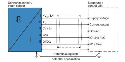
Output signal:  $I_{OUT} = 4 \dots 20 \text{ mA}$ , capable of parameterization Operating voltage range: +Vs = 18 to 30 VDC
