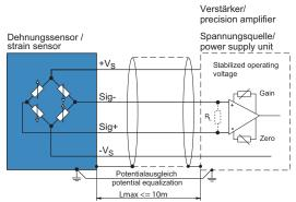
Output signal typical: Sig+ / Sig- = ±1.1 mV/V (the measured value is indicated on the sensor)
