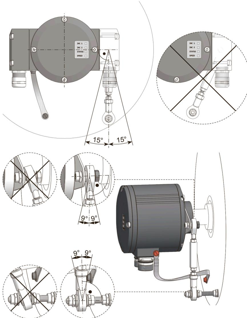
a) Mount the torque arm in a way that the shift towards the vertical encoder axis does not exceed  $15^\circ$  to the left or right.
