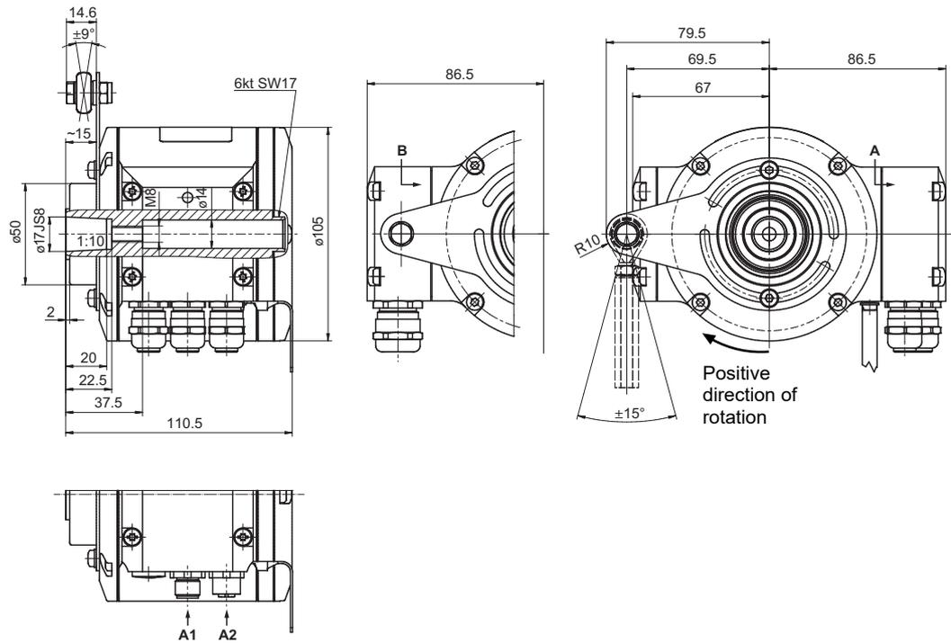
III. 16: Cone shaft dimensions (in mm unless specified otherwise)
