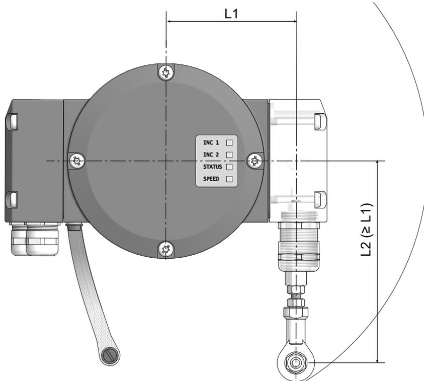
L1 Vertical distance of the torque arm towards the encoder center in mm
