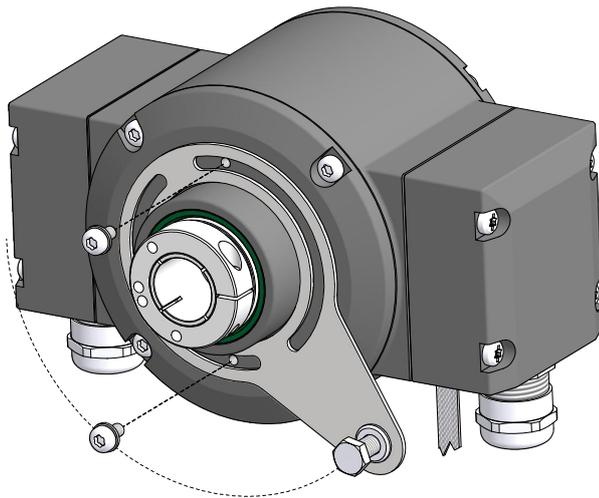
c) Move the torque support to the desired position.
