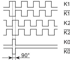
**7.3 Ausgangssignale POG 90 ... N (Sonderversion mit 180° elektrisch langem Nullimpuls)****7.3 Output signals POG 90 ... N (special version with zero pulse length of 180° el.)**
