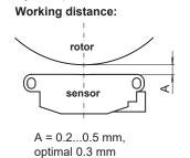
Use the distance band as s mounting tool for optimal gap (0.3 mm) between sensor and rotor.
