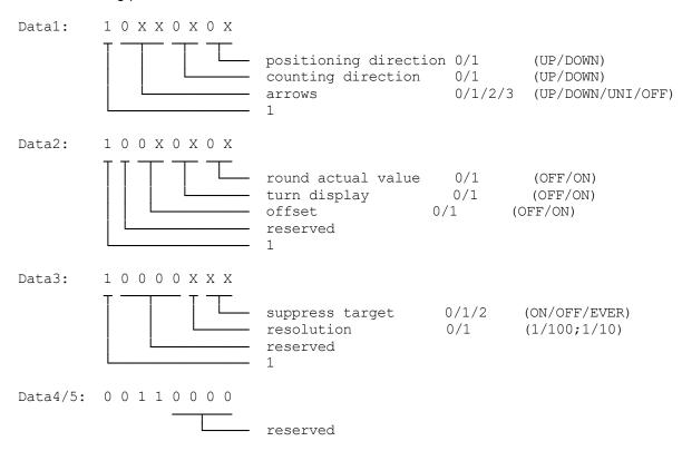
**Important:** Only the bits marked 'X' may be altered. The permanent parameters "1" and "0" must not be altered since this might create a control token ( tokens < 20h) what is not permitted in ASCII protocol.
