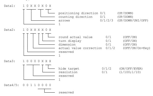
**Important:** Only bits marked 'X' may be altered. The permanent parameters "1" and "0" must not be altered since this might create a control token ( tokens < 20h) what is not permitted in ASCII protocol.
