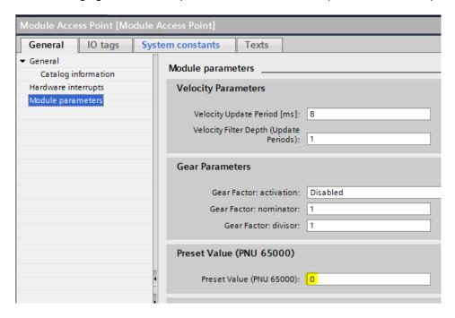
The preset value can be set to a value unequal 0. To do this no program, PLC function block or similar things are necessary. If one of the PROFIdrive telegrams 81 to 83 is used and a preset is triggered (in operation) the value in PNU 65000 is used as preset value.
