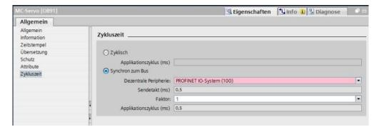
Enter process image partition (PIP) of clock-synchronous system function "MC-Servo" in the encoder property window.
