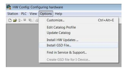
In the following dialogue please select the directory where to find the GSDML file which shall be installed. It is useful (but not necessary) to work with the program directory "...\Siemens\Step7® \S7Tmp".
