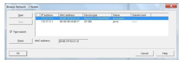
The MAC address ensures unique device recognition. Button "flash" will start the identified user's SF LED flashing for clear identification.
