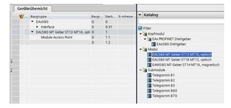
Select the requested submodule (telegram) and drag from hardware catalog to drop in subslot 1.2 (e.g. telegram 860).
