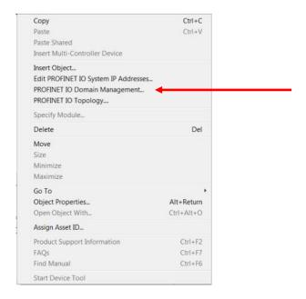
In the following screen "Domain Management" enter the "Sync domain" name or keep the default. For IRT Class 3 only enter the send clock here.
