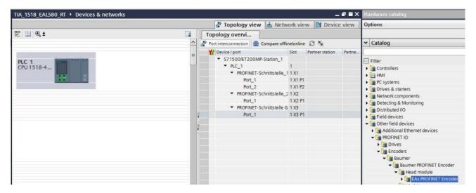
Use the mouse to drag head module "EAx580 encoder" from the hardware catalog for drop in PLC (framed slot). Next, use the mouse to draw the required connections between PLC and encoder ports.
