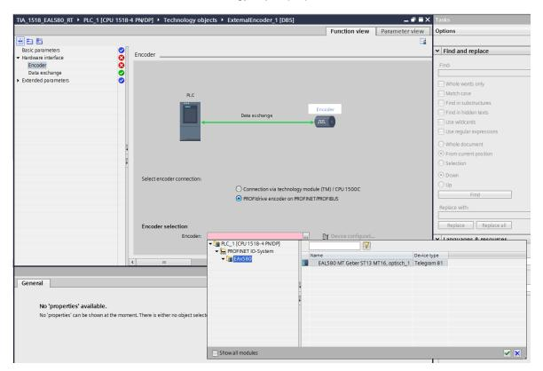
Window "data exchange" adopts telegram type, singleturn resolution, total number of revolutions as well as the telegram's bit number in both position values.
