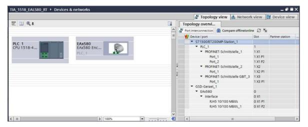
To execute topology planning use the mouse to drag a connection between the selected ports and bus users.
