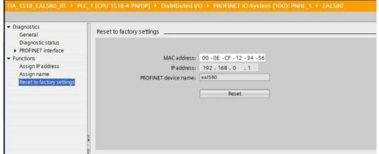
"Reset" will delete entire the customer configuration including device name and IP. MAC ID and serial number will remain. Switch the encoder off and on after factory setup.
