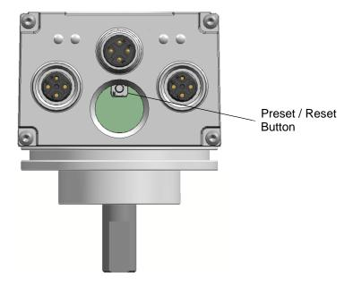
Depending on the current operating state the push button has a different functionality:
