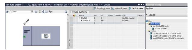
Select module in the hardware catalog (your encoder, e.g. "EAL580 MT Encoder ST13 MT16, optical") and drag and drop in slot 1 below "Interface".
