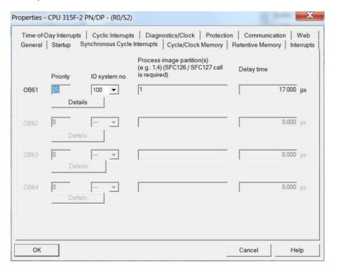
A click on button "Details" provides OB61 properties. Process image partition 1 is assigned to OB61.
