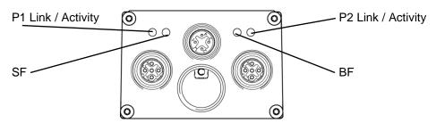
BF LED is red after encoder is powered on and red flashing for the time communication with the PROFINET PLC is being established. During connection establishment the BF LED is flashing red.
