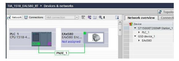
Clicking "not assigned" provides the available controller connections. After having selected the connection (in the "PLC\_1.PROFINET-interface\_1") the encoder assigns to the PLC.
