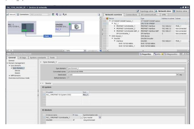
Enter selected synchronization clock in "Sync-Domain\_1". The selected clock will be applied by PLC and each device within this sync domain.
