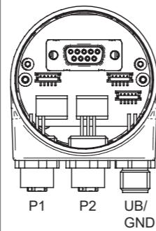
An optimized connection between encoder case and the braided shield of the connection cable is only achieved by the braided shield being placed generously onto the connector and the nut being secured firmly.
