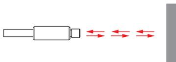
Diffuse sensors evaluate the intensity of light reflected by the object. One and the same sensing head accommodates both transmitter and receiver.
