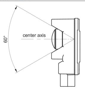
Objects within a rotational cone of  $\pm$  30  $^{\circ}$  may be picked up by the sensor depending on position and/or surface properties. When mounting behind a cover material properties and thickness must be taken into account to avoid excessive damping of the signal. Coatings containing metal must be avoided. The effect of objects in the defined free area must be verified in the application. Loose objects should be avoided.
