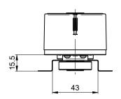
Through hollow shaft, flange socket M23
