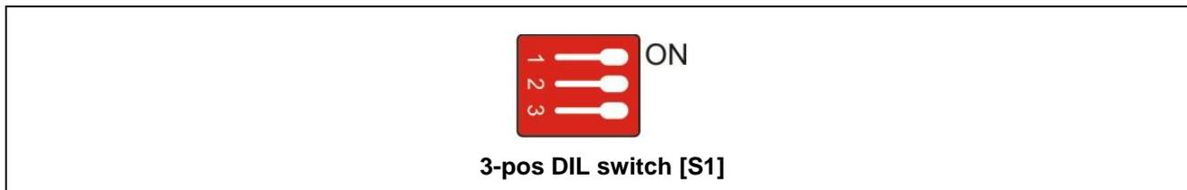
The DIL switch is used to set the operation state of the monitor:
