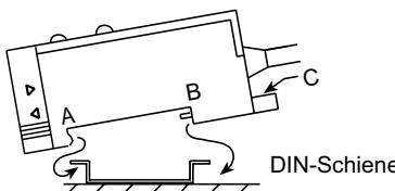
Mount the amplifier on the original bracket (supplied with amplifier) or the DIN rail.
