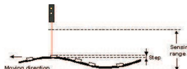
The desired height difference has to be first taught. Because the sensor only memorizes the difference, normally the absolute distance to the object is not relevant for the teach-in. The smallest teachable difference depends on the sensing distance (see diagram).
