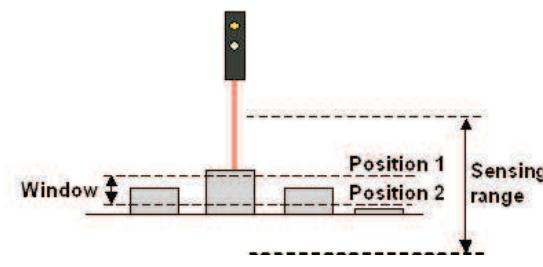
The two thresholds of the window have to be first taught. The smallest teachable window depends on the sensing distance (see diagram).
