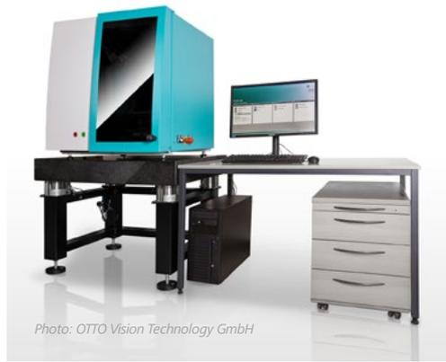
Two 12 megapixel Baumer CX series cameras used as stereo cameras acquire the images to create the 3D image. The optional motorized object frame allows for a full 3D scan from top and below. Optionally with vibration-isolated laboratory table.
