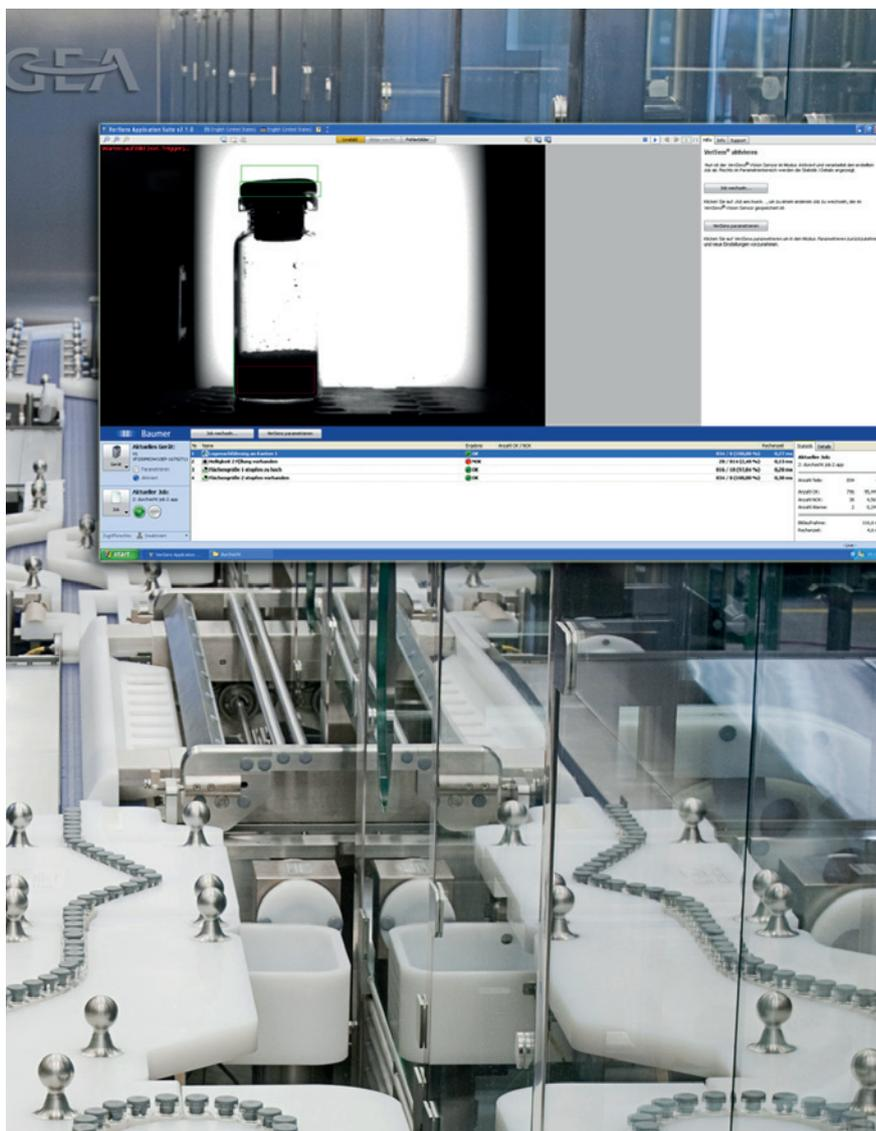
*The inspection tasks (jobs) for the simultaneous closure and level control of the vials are configured in the user-friendly VeriSens® software. The jobs can be selected according to vial size.*
