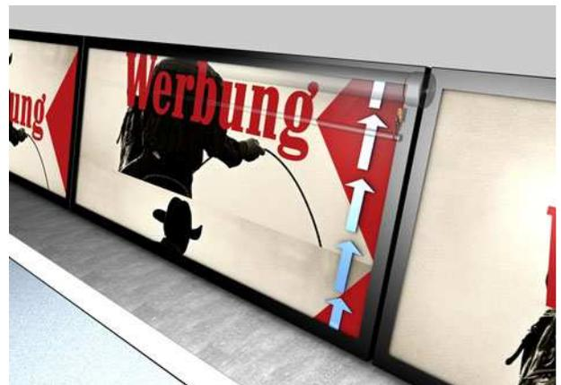
Figure 4a: A diffuse sensor with intensity difference detects print marks on strip advertising
