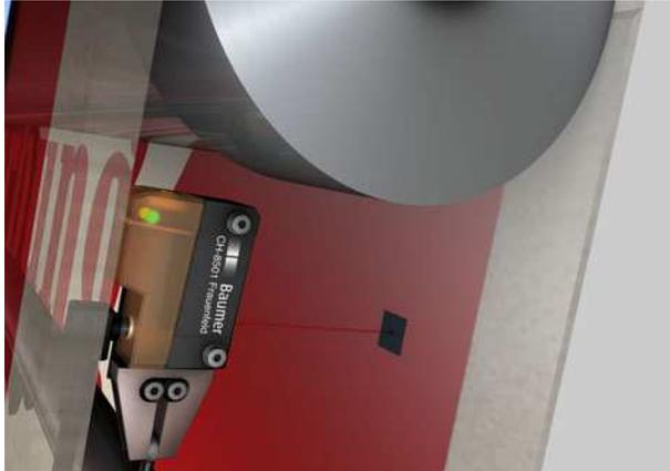
*Figure 4b: A diffuse sensor with intensity difference detects print marks on strip advertising (detailed view)*
