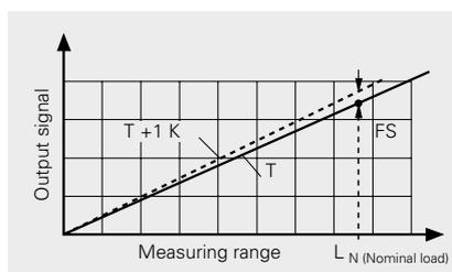
The largest temperature coefficient (TC) of output range is the largest variation in output range which occurs during a change in temperature by 1 Kelvin. It is expressed in percent of FS\*) per Kelvin.
