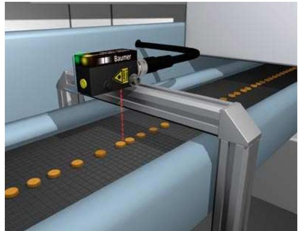
Figure 2: Reliable detection of small components on a conveyor belt using a laser sensor
