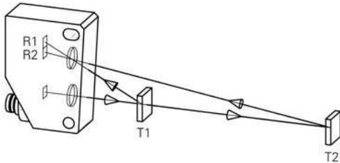
Figure 3: The principle of background suppression
