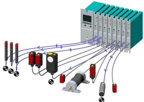
*Fig. 3 IO-Link-enabled and conventional sensors can be used together on one master.*
