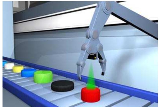
*Fig. 6 An ultrasonic sensor is mounted to a gripper and used for color-independent distance measurement.*
