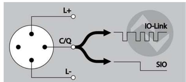
*Fig. 2 In IO-Link mode, serial data can be transmitted by way of the switching output.*
