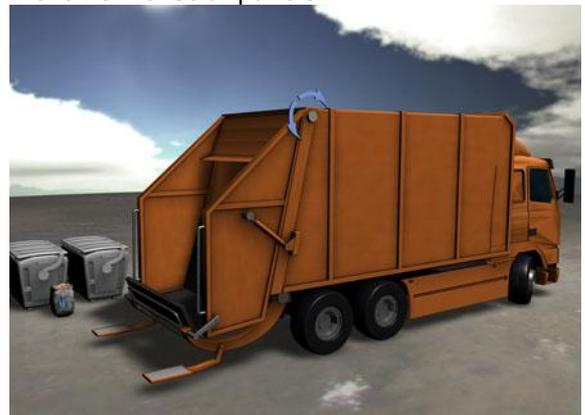
*Fig. 6: Using magnetic rotary encoders to control the inclination angle of dump truck loading equipment*
