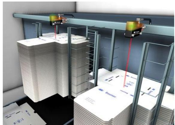
*Fig. 2: Using photoelectric sensors to measure stack height in the printing or packaging industry*
