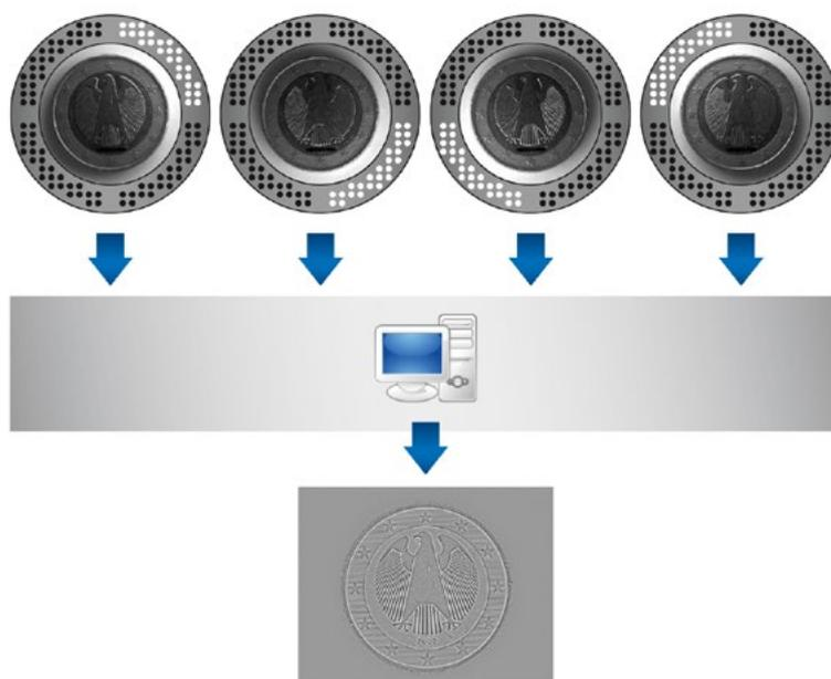
In shape from shading applications, the inspected object is being successively illuminated from four different directions while taking one gray-scale image each. The evaluation of the resulting surface shadings provides information about the surface quality.
