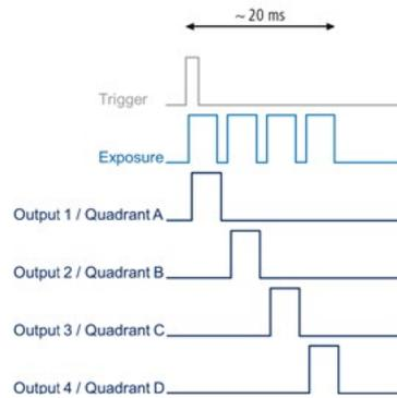
Example sequencer timing for triggering four lighting units (output 1 to 4) straight by the camera (e.g. VCXG-13M.I) without the need for an external lighting controller.
