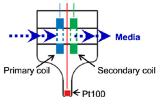
Figure 1: Schematic presentation of the inductive measuring principle
