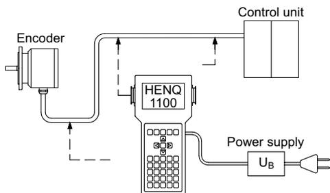
Error analysis through a step-by-step check of the test signal at various points in the signal path
