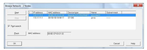
The MAC address serves as a unique identifier. When clicking the button "Flash" the highlighted device will flash its status-LED so it can be found easily amongst other devices.
