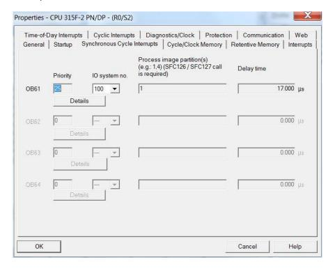
A click on button "Details" provides OB61 properties assigned sub-process image 1.
