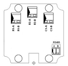
Fig. 18: DSL.E terminal assignments
