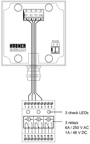
Fig. 20: Connections for DS 93 R
