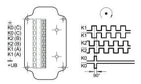
Fig. 17: POG/HOG terminal assignments
