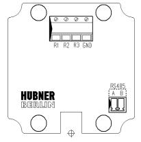
Fig. 19: DSL.R terminal assignments
