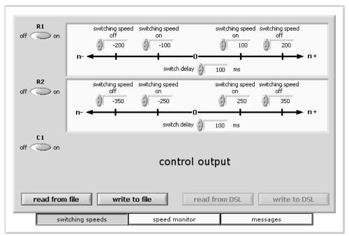
Fig. 11: "Switching speeds" register for DSL.E
