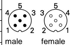
Terminals with the same significance are internally connected and identical in their functions. Max. load on the internal terminal connections UB-UB and GND-GND is 1 A.
