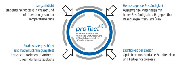
Fig. 5 Baumer sensors with proTect+ provide outstanding impermeability and an extended lifetime
