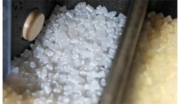
*Figure 5: Even when things get hot such as in this hot melt adhesive processing unit, capacitive sensors are suitable for fill level monitoring.*
