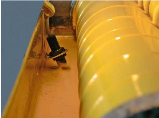
*Figure 4: The fill level in even large color tanks can also be monitored by capacitive sensor.*
