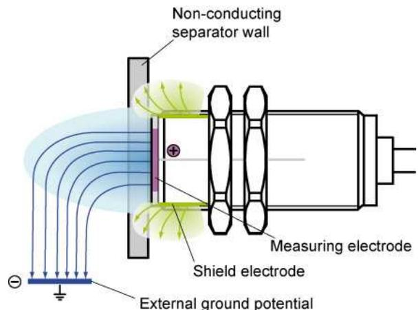
Figure 3: With the new sensors, the ground electrode in the form of the medium or a grounded object is located outside the sensor itself, thus offering a significant increase in the sensing distance.
