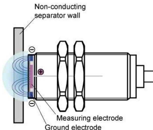
Figure 2: Previously employed shielded mount capacitive sensors possess only a limited sensing distance.
