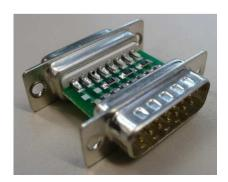
Figure 3: Terminating resistor adapter
