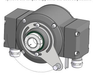
d) Tighten the Torx screw with 2-3 Nm.
