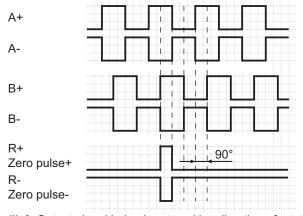
III. 9: Output signal behavior at positive direction of rotation
