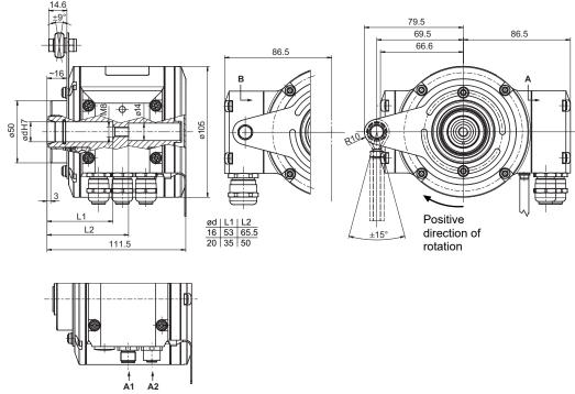
III. 14: Dimensions of blind hollow shaft in mm (unless specified otherwise)
