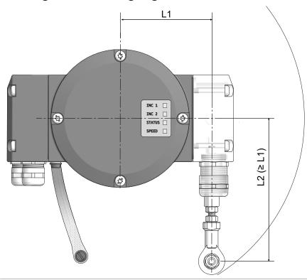
L1 Vertical distance of the torque arm towards the encoder center in mm L2 Torque arm length (≥
