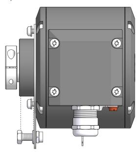
b) If required, you may remove the Torx screws completely for turning around the torque plate. Then carefully screw the Torx screws back in, but do not tighten already.
