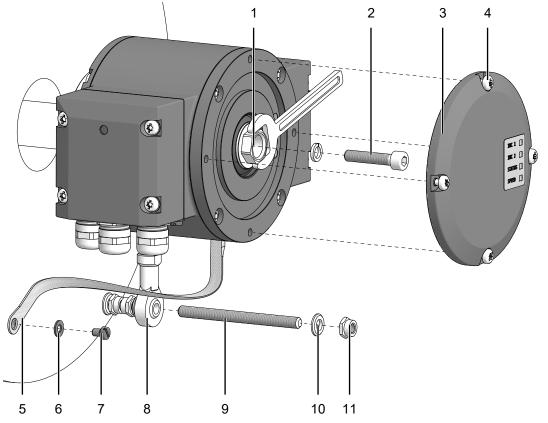
Blind hollow shaft or cone shaft with Cheese-head screw M6x30 mm (ISO wrench flat SW 17 mm 4762) 3 Cover 4 Torx/slotted head screw M4x10 mm (DIN 7964) 5 Washer B6.4 for grounding strap (ISO Grounding strap 7090) 7 Cheese-head screw M6x8 mm for Torque arm 8 grounding strap (ISO 1207) 9 Threaded rod M6, variable length ≤ 210 Washer B6.4 (ISO 7090) 10 mm
