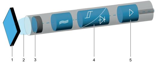
III. 1: Inductive sensor: Function principle (schematic representation)
