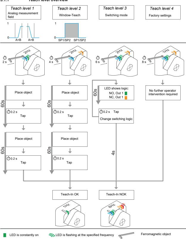
0.2 s Touch the sensor's teach field with a ferromagnetic tool and hold for the specified time
