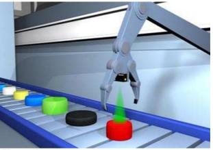
Fig. 6 An ultrasonic sensor is mounted to a gripper and used for color-independent distance measurement.
