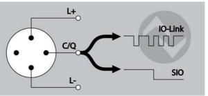
Fig. 2 In IO-Link mode, serial data can be transmitted by way of the switching output.
